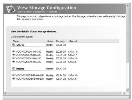
Figure 27. View Storage Configuration (MediaShield)
