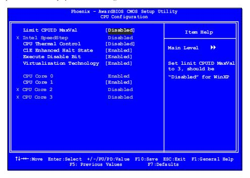
Figure 11. CPU Configuration Menu
