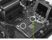
Align notches with notches on the CPU
